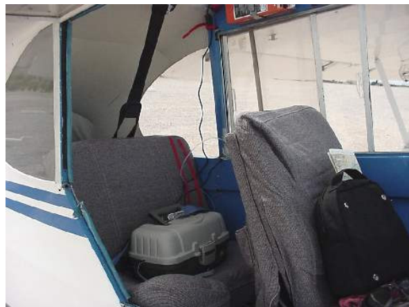
Figure 3-6. Sampler Mounting in Back Seat of Tow Aircraft
